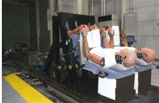
Vertical impact testing, simulating an ocean-based impact and resulting rebound and landing on the water
