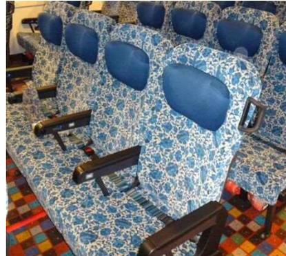
The renewed passenger seating, equipped with specially-designed two-point retractable seat belts
